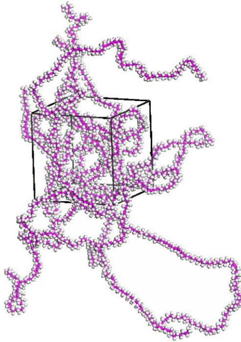
Fig. 5. Shown is a polythene system consisting of 4808 atoms. The pink backbone consists of carbon atoms while the hydrogen atoms are rendered in white.
