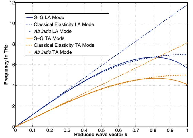
FIG. 1 (color online). Shows the comparison of phonon dispersion curves of copper (Cu) predicted by strain-gradient elasticity (S-G modes) and classical elasticity to those obtained by *ab initio* calculations for the transverse acoustic (TA) and longitudinal acoustic (LA) modes along  $\mathbf{k} = [100]$ .
