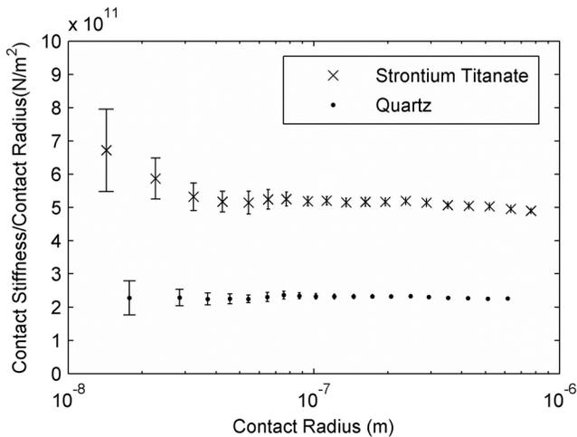
FIG. 1. Variation of contact stiffness of SrTiO<sub>3</sub> as a function of contact radii.
