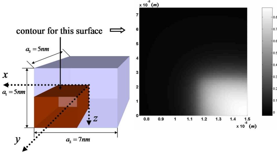
FIG. 6. (Color online) Strain gradient results for dilation strain of cuboidal quantum dot. Dilation strain is normalized as  $\text{Tr}(\varepsilon_{ij})(2\mu + \lambda)/P^m$ . Light area represents high dilation. Internal length scale is  $l' = 0.82$  nm.
