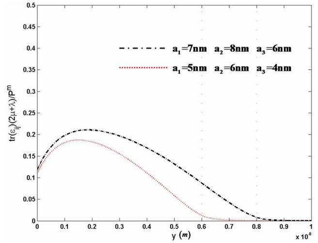
FIG. 14. (Color online) Strain dilation along  $y$  axis.
