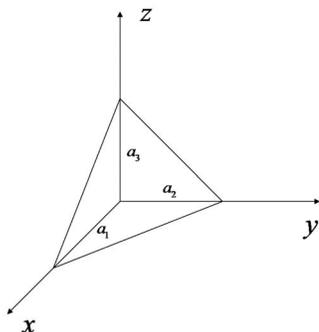
FIG. 13. Schematic figure of orthogonal polyhedral QD.
