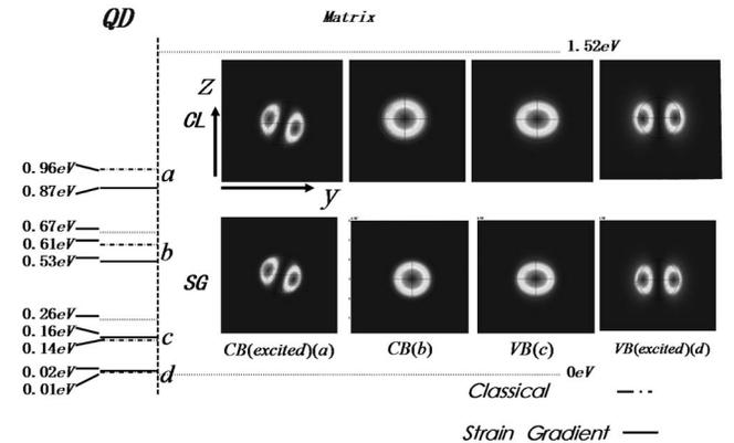
FIG. 19. Band energies and carrier density  $|\psi|^2$  for QD with radius equal to 5 nm. The central areas (dark gray) indicate higher numbers for the contour plot for carrier density. These results are for a slice of the  $y$ - $z$  plane.
