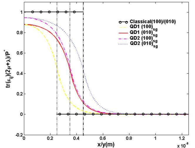
FIG. 7. (Color online) Normalized strain dilation is plotted for two directions on the crossing plane  $z=0$ . The subscript “sg” indicates strain gradient while “cl” indicates classical. Vertical dotted lines mark the boundary of QD at two directions ( $x$  and  $y$ ). QD1’s size is  $a_1 = 5$  nm,  $a_2 = 7$  nm, and  $a_3 = 5$  nm. QD2’s size is  $a_1 = 7$  nm,  $a_2 = 9$  nm, and  $a_3 = 7$  nm.
