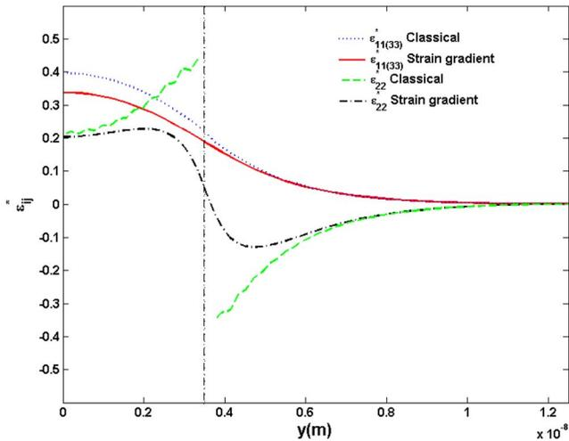
FIG. 8. (Color online) Strain components  $\epsilon_{11}$  and  $\epsilon_{33}$  of cuboidal QD with  $a_1=5$  nm,  $a_2=7$  nm, and  $a_3=5$  nm. Vertical dotted line is the boundary of the QD. The plot is along (010).
