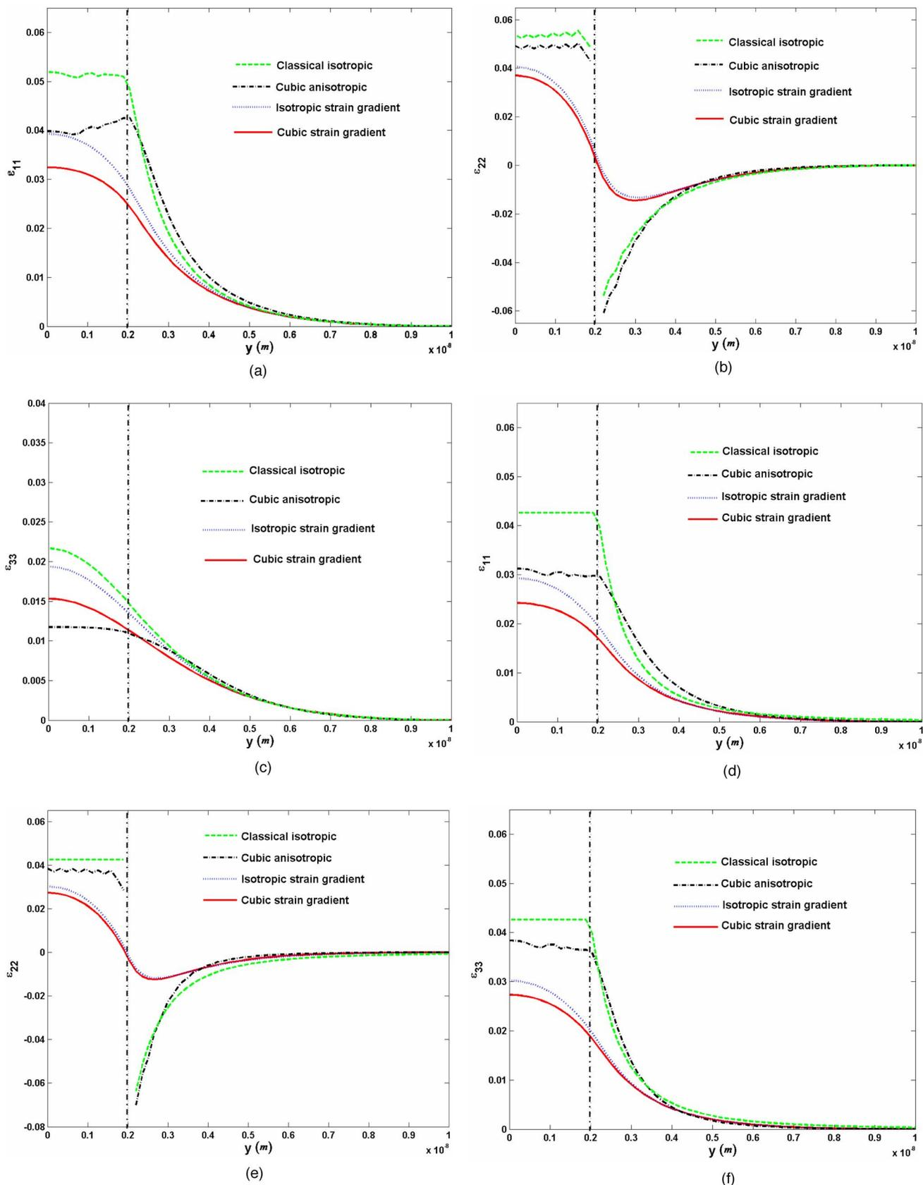
FIG. 16. (Color online) Strain component of finite cylinder QD for different cases (a)  $\epsilon_{11}$ , (b)  $\epsilon_{22}$ , (c)  $\epsilon_{33}$ . Strain components of sphere QD for different cases (d)  $\epsilon_{11}$ , (e)  $\epsilon_{22}$ , (f)  $\epsilon_{33}$ . (In the classical isotropic case,  $\epsilon_{33}$  should be equal to  $\epsilon_{11}$  due to symmetry, which is indicated here. However, it is different for the anisotropic case.)
