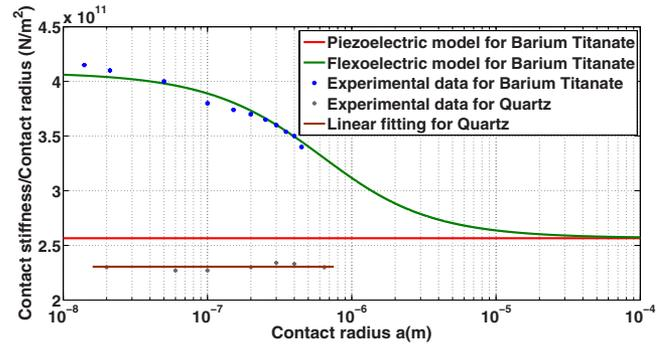
FIG. 2. (Color online) Variation in the ratio of the contact stiffness and contact radius as a function of contact radius. Experimental results for both BaTiO<sub>3</sub> and Quartz are plotted along with the results from the flexoelectricity and classical piezoelectricity based models.
