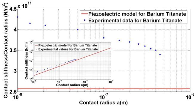
FIG. 1. (Color online) Variation in the ratio of the contact stiffness and contact radius with respect to the contact radius  $a$  for BaTiO<sub>3</sub>. The inset graph plots the contact stiffness vs radius.
