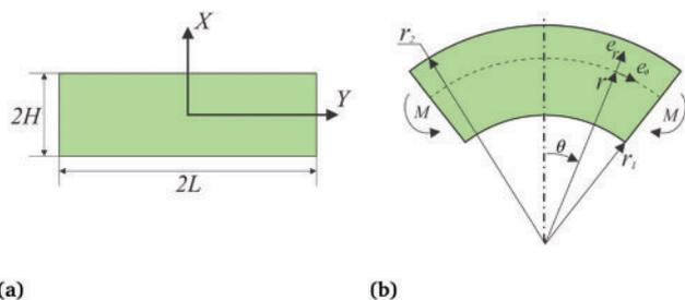
Fig. 7 Schematic of the coordinate systems used in the reference and current configurations. (a) Cartesian coordinates are used in the undeformed block. (b) A cylindrical coordinate system is employed for the deformed block.
