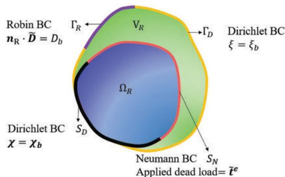
Fig. 3 Continuum deformable body in the reference configuration and applied boundary conditions.
