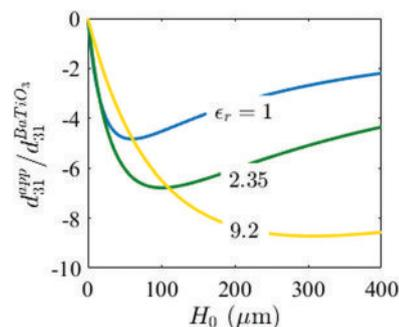
Fig. 17 Apparent piezoelectric coefficient of a polymer film with embedded dipoles attached to another material free of dipoles with thickness  $H_0$ .
