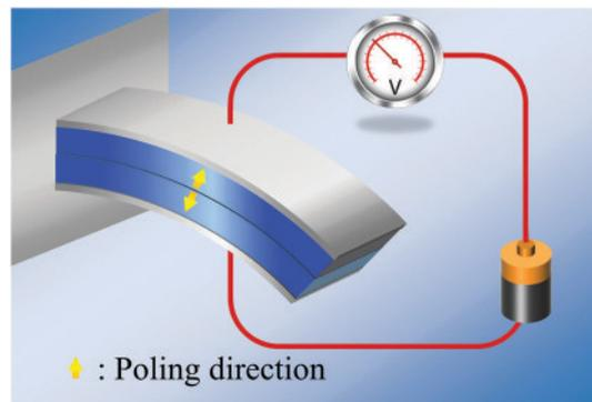
Fig. 1 Bending piezoelectric actuator is based on the so-called  $d_{31}$  piezoelectric effect. Typically, this actuator is made of two layers of piezoelectric materials with opposite poling directions. Generation of displacement in opposite directions in response to applied electric field bends the structure.
