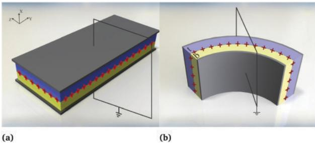
Fig. 19 A composite block made of two layers with two different dielectric materials and a layer of charge is inserted between two layers. (a) Undeformed configuration. (b) Deformed configuration.
