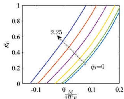
Fig. 13 Effects of external charges on the curvature of the block for  $\alpha = 0.5$ .
