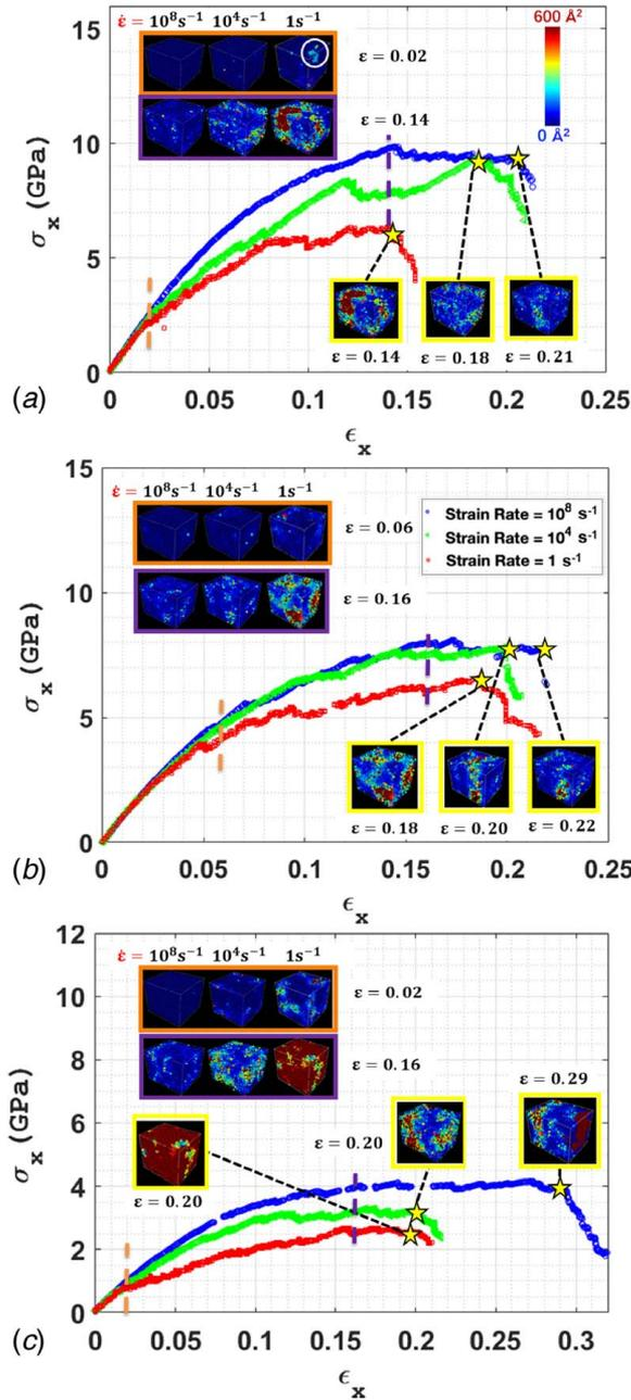
**Fig. 3 Stress–strain curves at different loading rates for (a)  $\text{LiSi}_2$ , (b)  $\text{LiSi}$ , and (c)  $\text{Li}_{15}\text{Si}_4$ . (All the curves share the same legend shown in (b) and all the snapshots share the same color bar shown in (a).)**
