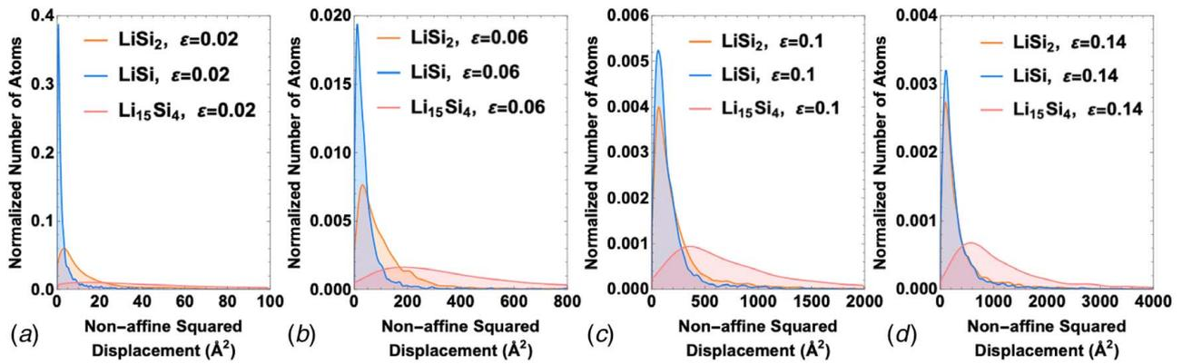
Fig. 7 Smoothed histogram plot of normalized atom number at varying non-affine squared displacement values for  $\dot{\epsilon} = 1 \text{ s}^{-1}$ . Plots denote the strain stage of (a) 0.02, (b) 0.06, (c) 0.1, and (d) 0.14, respectively.
