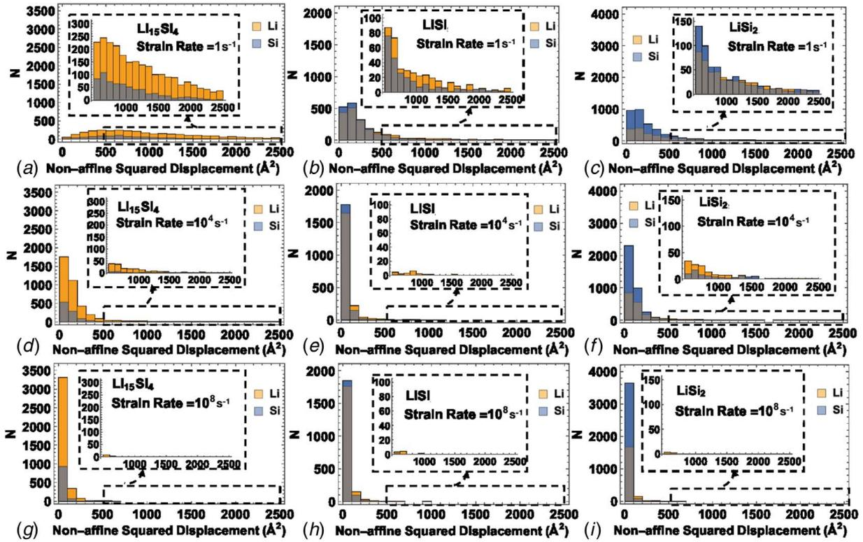
Fig. 5 Number of atoms for each non-affine squared displacement range at the strain of 0.14. Top, medium, and bottom row are for the strain rate of  $1 \text{ s}^{-1}$ ,  $10^4 \text{ s}^{-1}$ , and  $10^8 \text{ s}^{-1}$ , respectively, and left, middle, and right columns correspond to  $\text{Li}_{15}\text{Si}_4$ ,  $\text{LiSi}$ , and  $\text{LiSi}_2$  structures, respectively.
