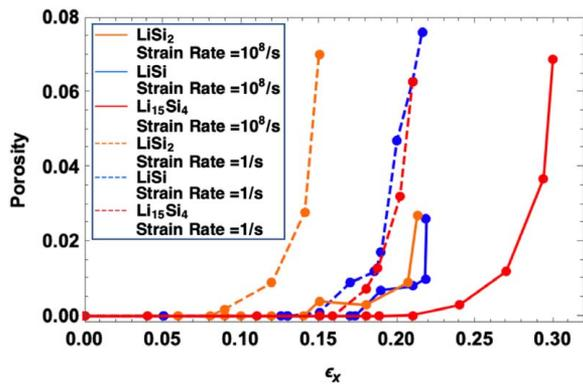
**Fig. 10 Porosity variation versus strain for  $\text{LiSi}_2$  (orange lines),  $\text{LiSi}$  (blue lines), and  $\text{Li}_{15}\text{Si}_4$  (red lines) at the strain rate of  $1 \text{ s}^{-1}$  (dashed lines) and  $10^8 \text{ s}^{-1}$  (solid lines)**
