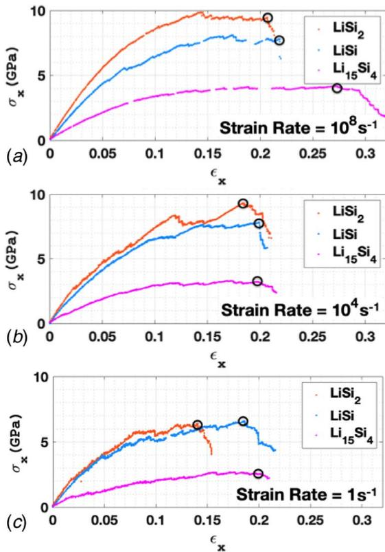
Fig. 6 Stress-strain curves for ABC simulations at the strain rate of (a)  $10^8 \text{ s}^{-1}$ , (b)  $10^4 \text{ s}^{-1}$ , and (c)  $1 \text{ s}^{-1}$ . Orange, blue, and pink correspond to  $\text{LiSi}_2$ ,  $\text{LiSi}$ , and  $\text{Li}_{15}\text{Si}_4$ , respectively. Here, points marked with circles denote the initiation of fracture.
