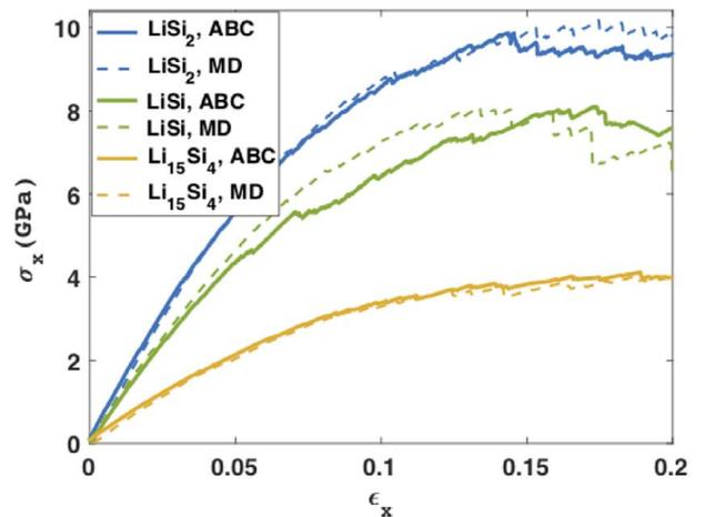
Fig. 2 Comparison of MD (dashed lines) and ABC (solid lines) uni-axial stress-strain curves for tensile test of same initial sample (created under quenching rate of  $4.4 \times 10^{11} \text{ K s}^{-1}$ ) and the strain rate of  $10^8 \text{ s}^{-1}$ . MD stretch was conducted at a temperature of 1 K. Here, blue, green, and yellow colors refer to  $\text{LiSi}_2$ , LiSi, and  $\text{Li}_{15}\text{Si}_4$  structures accordingly.
