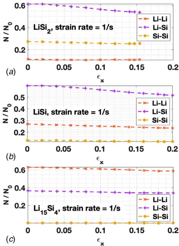
Fig. 8 Normalized bond number variation of loading at a strain rate of  $1 \text{ s}^{-1}$  for (a)  $\text{LiSi}_2$ , (b)  $\text{LiSi}$ , and (c)  $\text{Li}_{15}\text{Si}_4$
