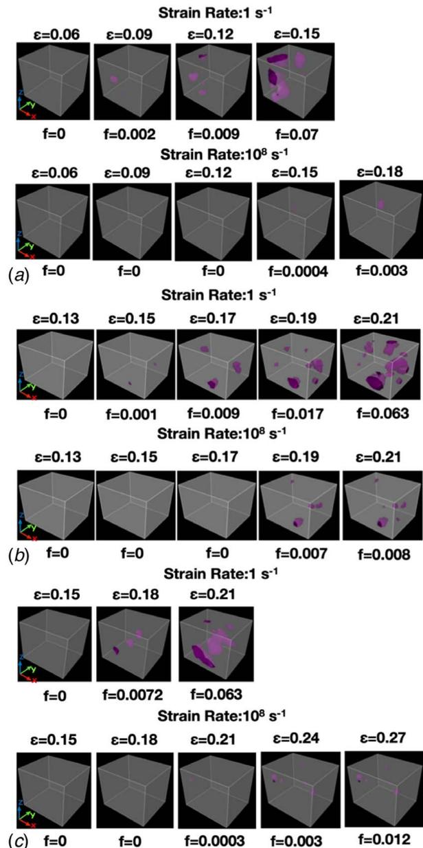
Fig. 9 Void nucleation of (a)  $\text{LiSi}_2$ , (b)  $\text{LiSi}$ , and (c)  $\text{Li}_{15}\text{Si}_4$  at a strain rate of  $1 \text{ s}^{-1}$  (top lines) and  $10^8 \text{ s}^{-1}$  (bottom lines)
